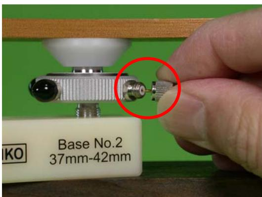
Then connect the **output cable** into **the sensor**. Insert the center pin of the **output cable** into the center hole of the **output connector**.
